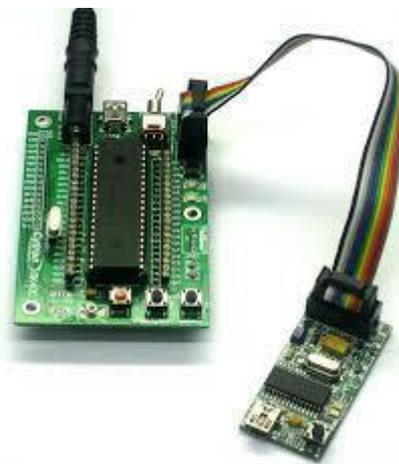
**Figure 4.** PIC microcontroller kit
