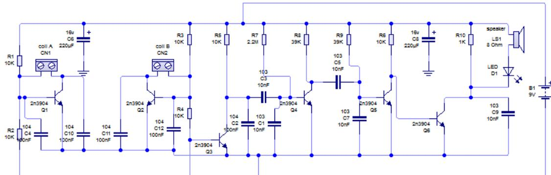
**Figure 1.** BFO metal detector circuit
