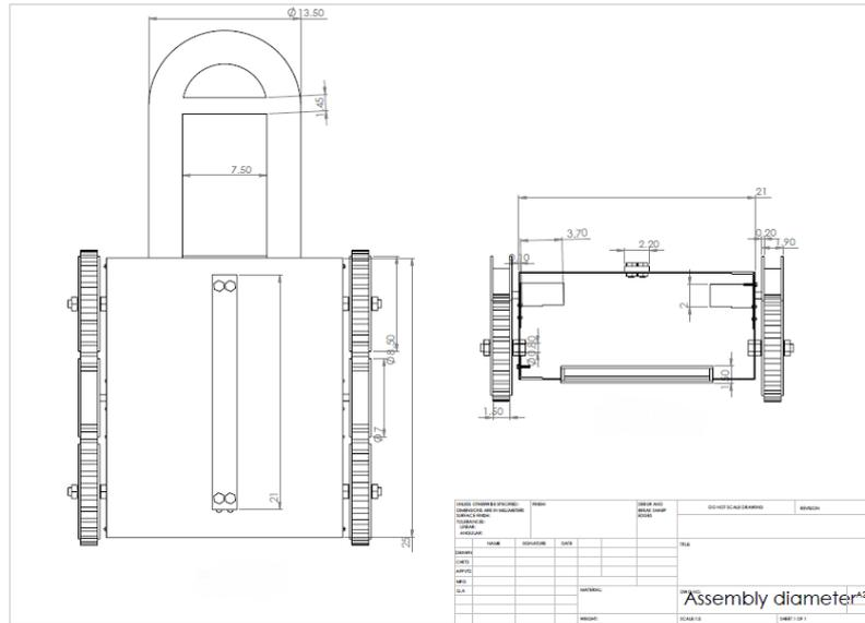
**Figure 6.** Caterpillar wheel robot
