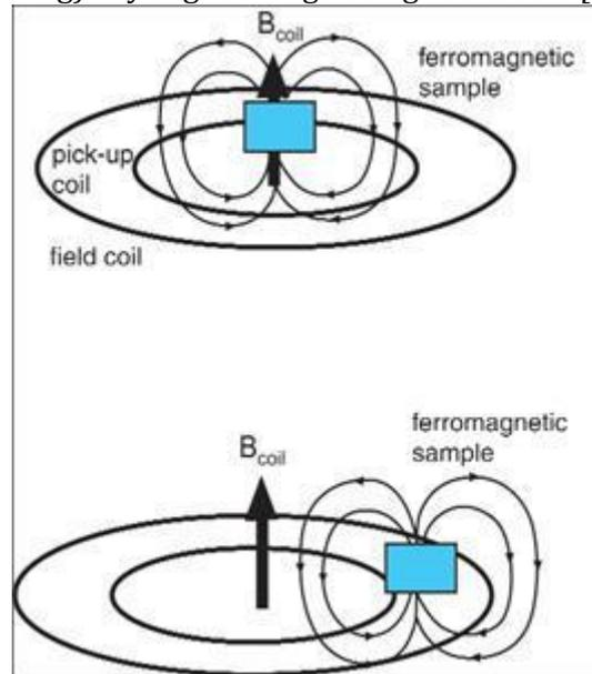
**Figure 2.** Example of pulse induction coil winding and their emf
